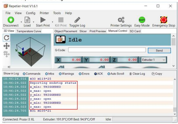
When the endstops are **not** pressed they should read as *Open*
