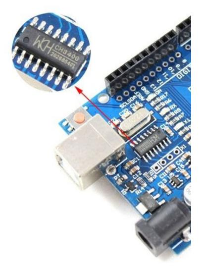
Download the CH340 driver, extract and install: <a href="http://www.diyelectronics.co.za/firmware/Software/Drivers/CH340%20Driver.zip">http://www.diyelectronics.co.za/firmware/Software/Drivers/CH340%20Driver.zip</a> NB if you have a CH340 chip and use Mac OS then please follow <a href="mailto:this.guide">this.guide</a>.
